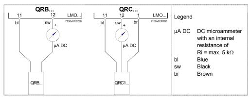
As an alternative to detector current measurement, the diagnostic tool OCI400 / ACS400 can be used. In that case, connection of a DC microammeter is not required.
